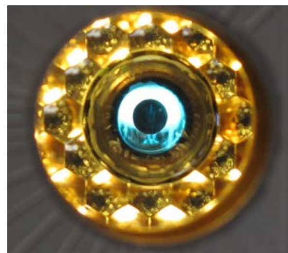
Top: The hohlraum target, pictured, measures about 10 mm long and about 6.4 mm in diameter. It contains the smaller fuel capsule. Credit: LLNL.
