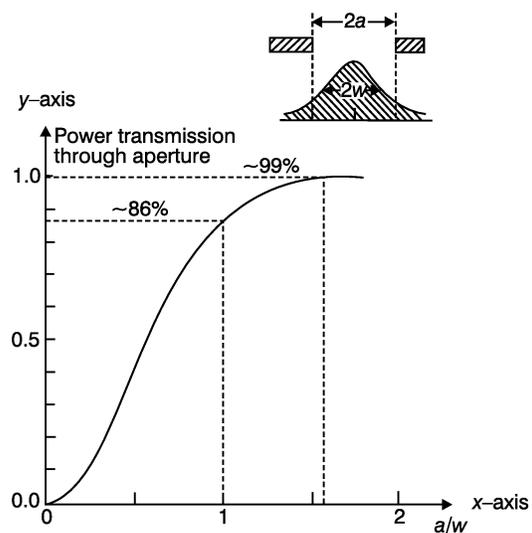
Power transmission of a TEM<sub>00</sub> cylindrical gaussian beam through a circular aperture, of diameter  $2a$ .
