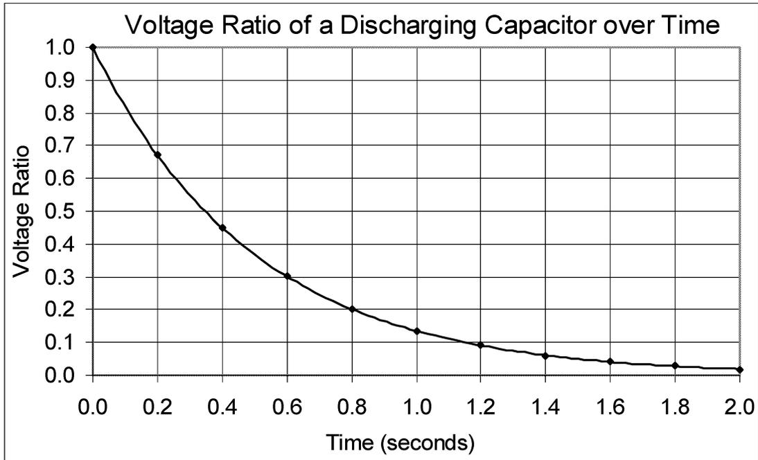
Initially the voltage ratio rapidly decreases, but as it approaches zero the decrease slows. We say that it approaches zero *asymptotically*. The rate at which it decreases is called the *time constant* ( $\tau$ ). It can be calculated by multiplying the resistance by the capacitance ( $R \times C$ ). Now we can rewrite the equation stated earlier:
